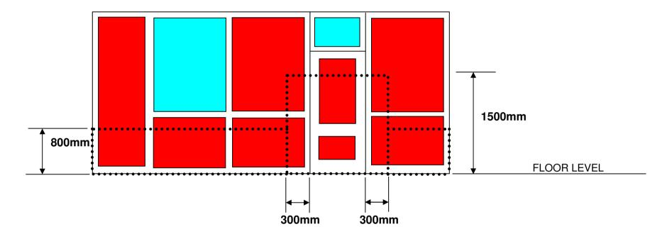
SAFETY GLAZING ZONES WITHIN THE DOTTED AREAS 800MM FROM FLOOR LEVEL (EXCEPT WITHIN 300MM OF A DOOR SEE BELOW) DOOR ZONES - WITHIN 300MM EACH SIDE OF A DOOR & WITHIN 1500MM FROM FLOOR LEVEL
